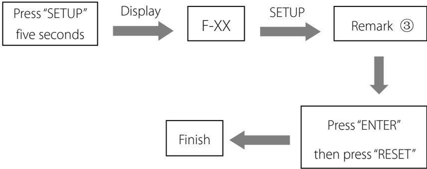
Remark ③: "xx" means working frequency ,press "SETUP" to select frequency, the scope for working frequency is 1-12 can be selected.
