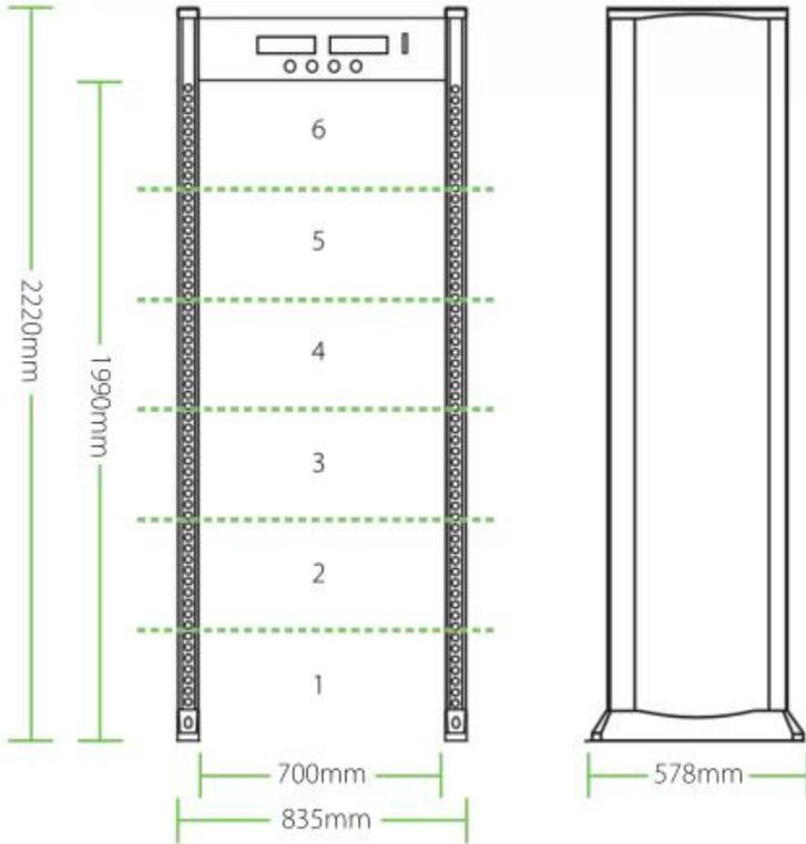
Input voltage: 100-240V, 50/60Hz      Power: 12W
