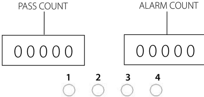
1. **ENTER:** confirm the data after adjusting, and change the single digit when setting the zone sensitivity level.
